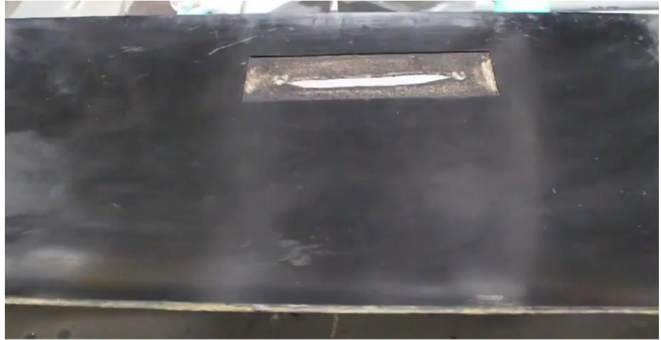
Figure 16. Damaged conveyor belt.
