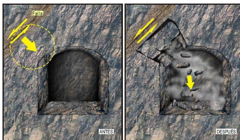
Figure 6,6: Problems of instability when the excavation advances in parallel and very close to a geological fault.
