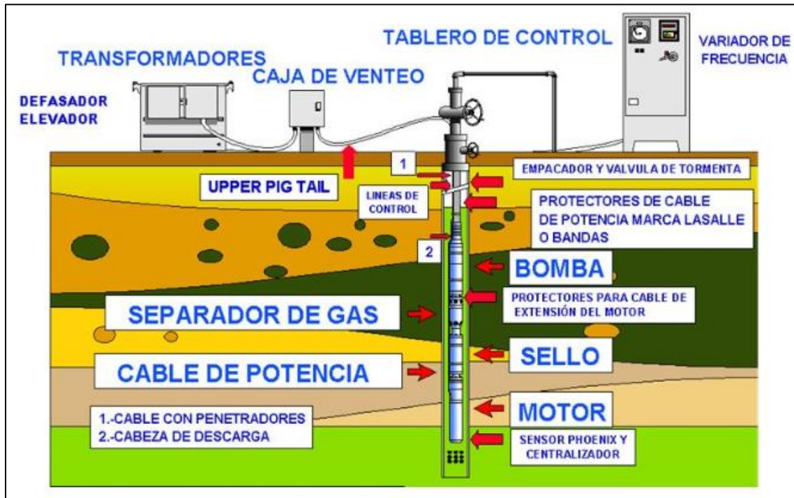
Figure 106. Surface and downhole equipment of an ESP system (E. Vargas).
