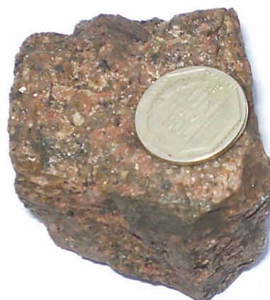
Figure 4. Medium grain biotitic granite (granular hipidiomorphic), incipient alteration (kaolin, sericite and chlorites).
