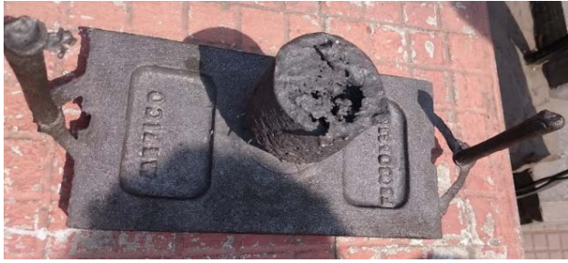
Drawn 2. Pieces obtained with the use of ceramic filters
