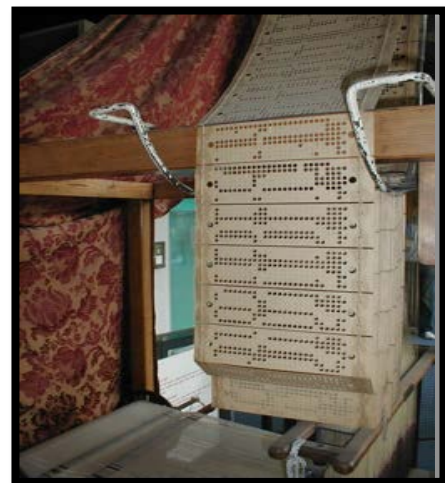
Fig. 2: Punch cards on a Jacquard loom
