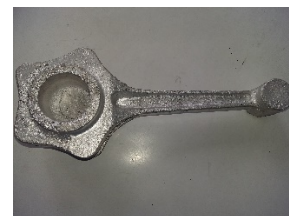
Figure 11. Connecting rod ( radial engine ) fused with respective faults, porosity, rechupes falling apart.
