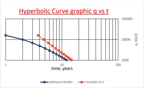
The data of the rate b / d have some variation since the solver works with discrete declination and the graphs with nominal declination.
